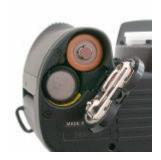
The CR123A batteries are inserted one at a time into the camera:
