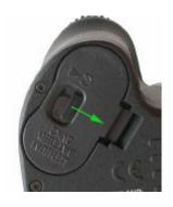
There's a yellow label in the battery compartment to help you remember the orientation of the batteries, and the silver piece on the hinged door also has + and – markings.
